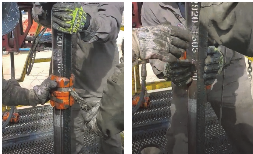
WWT Slider-Clamp During the Uninstall Process
