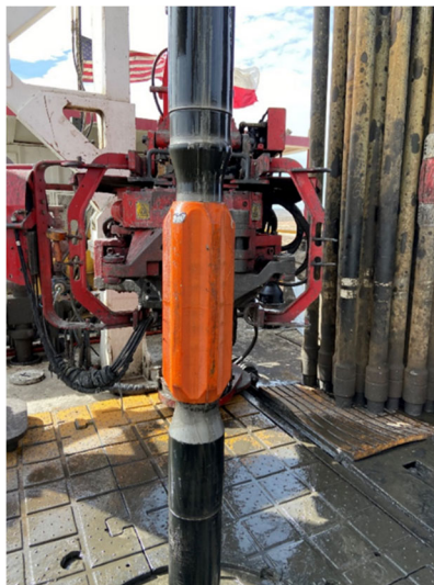
WWT Silencer Sub compared to typical tool joint wear after drilling curve section of the well.
