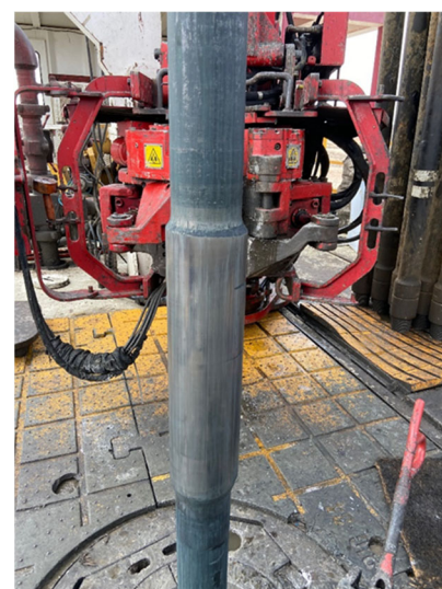
WWT Silencer Sub compared to typical tool joint wear after drilling curve section of the well.
