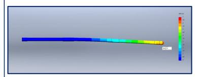
Image of FEA analysis showing approximately 6" downward deflection in a horizontal wellbore. This allows the shoe to locate and enter a low-side sidetrack regardless of casing orientation.
