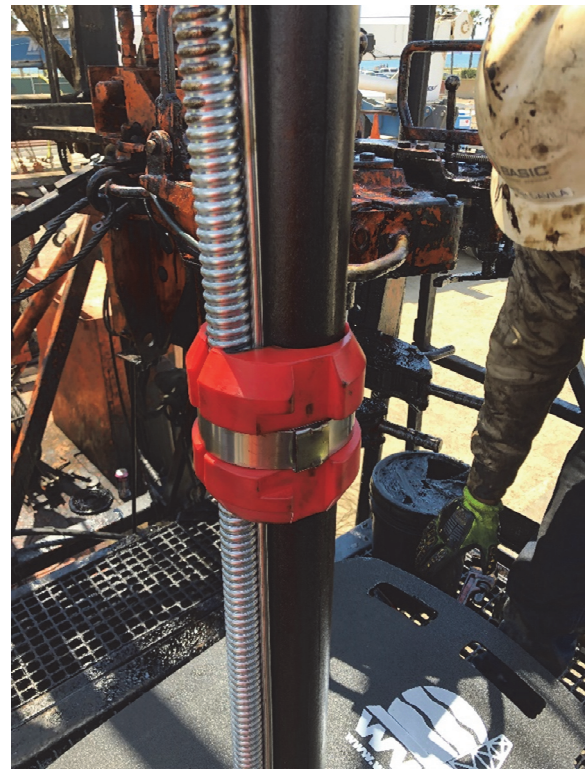
WWT Slider-Clamp low friction cable protector.
