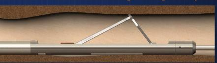
Figure 2 WWT Eccentric Link Gripper
