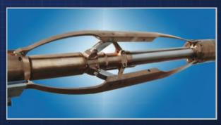
Figure 2 WWT Expandable Ramp Gripper assembly
