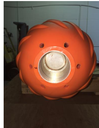
Photo showing the 9-5/8" JetGuide with closed center nozzle and outer ring of six jetting nozzles.
