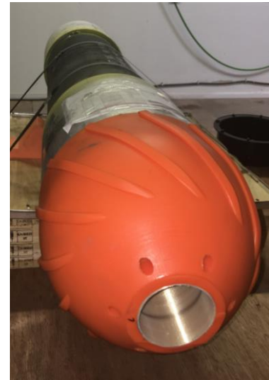
9-5/8" JetGuide with crossover just prior to being sent to the rig.
