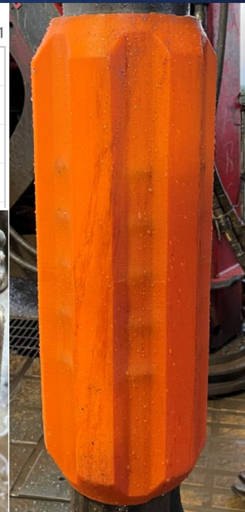
Silencer in good condition after reaching TD (drilled 12,398') Avg OD wear = 0.21".
