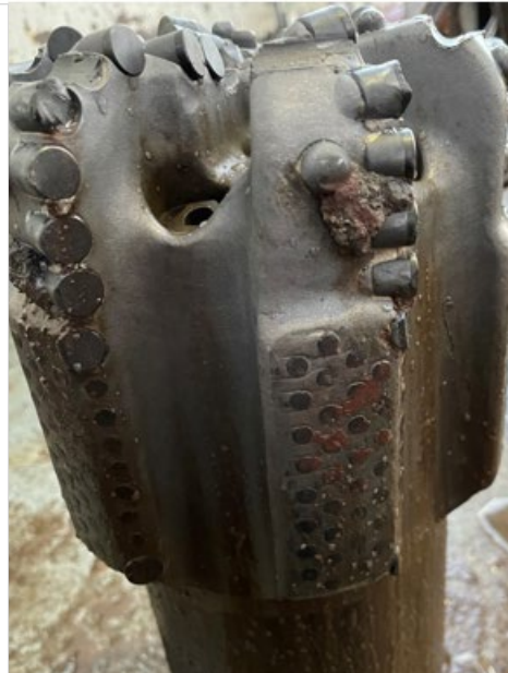
Bit after setting record length run. No wear to outer pads/shoulders.
