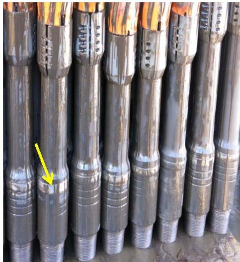
Figure 2: Tool joints with NRPs had visibly less wear, indicating stand-off was properly maintained.
