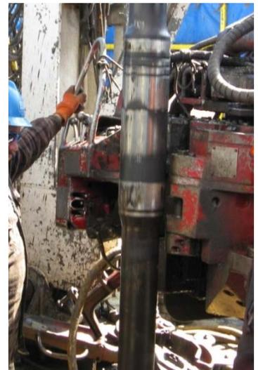
Figure 3: Unprotected tool joints were polished, indicating wear.
