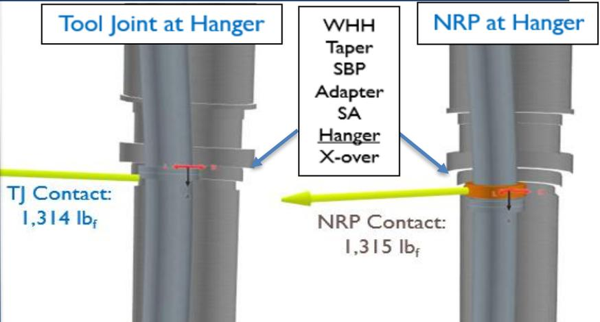
**Image 1.** Complete tool joint stand-off achieved while drilling with NRPs installed.
