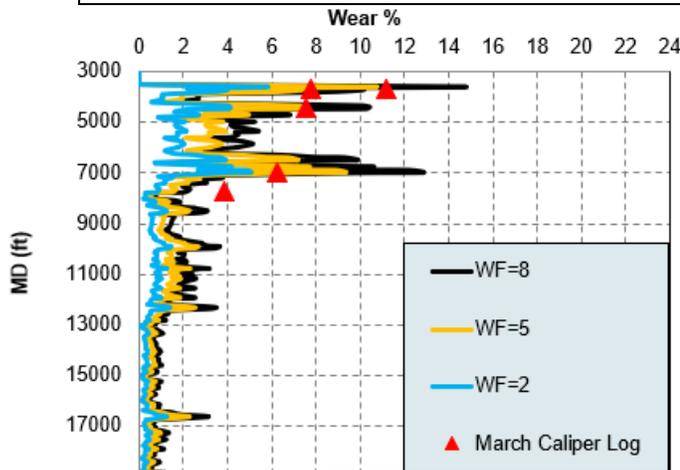
**Cumulative Wear After Drilling the last 2 Hole Sections
