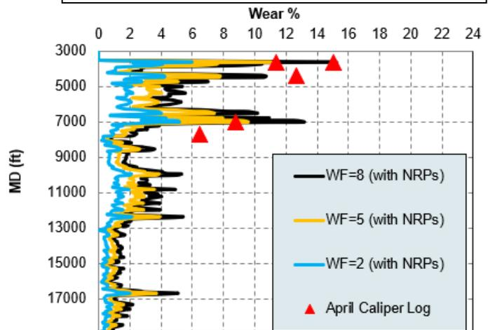
**Image 2.** Cumulative wear to the casing without NRPs vs with NRPs
