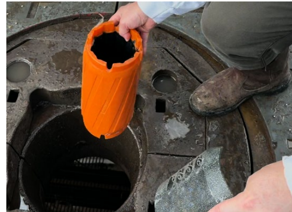
SS3-400-slim and 4" slim collar being thrown in the well
