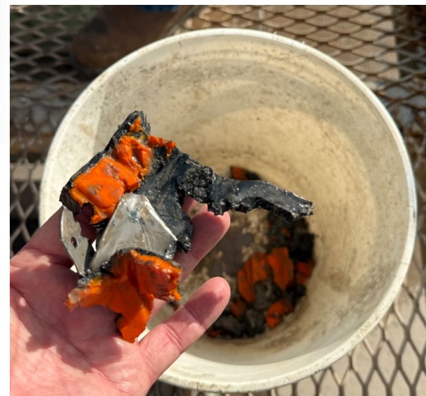
S4-400-slim-RS debris recovered on shakers
