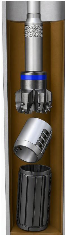
Illustration of the S4-400- slim-RS and 4" slim collar inside the hole
