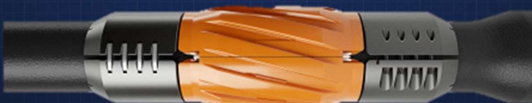
Figure 2: NRPs Clamp Onto the Drill Pipe Body to Mitigate Friction and Buckling to Decrease Torque and Drag.
